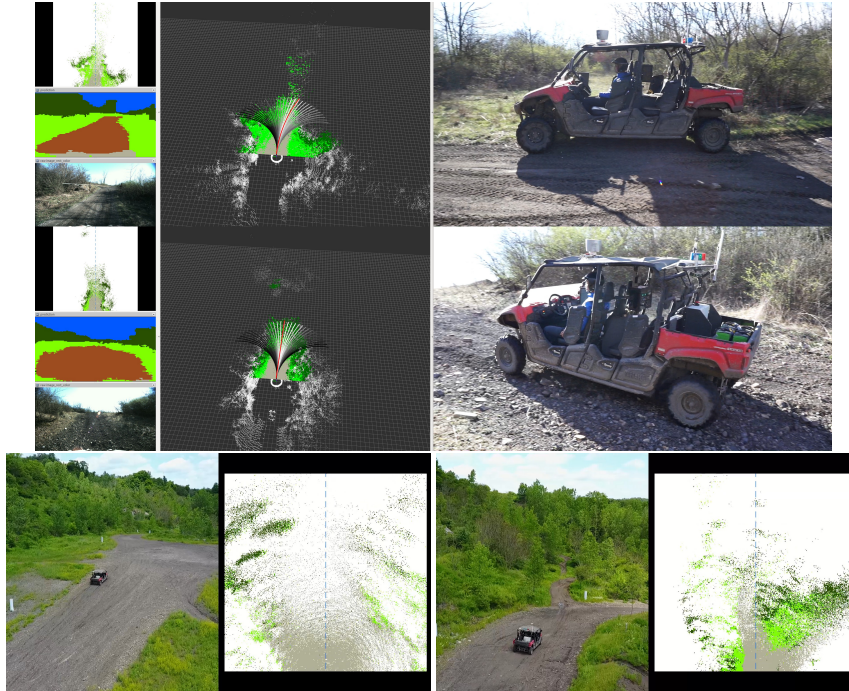
Fig. 10 Action shots of autonomous off-road driving in our testing site. In the first two rows, the left-hand side shows screenshots of the sensor data and map as seen from the vehicle. The last row shows aerial action shots with the right-hand showing the semantic map. Videos will be made available on the project page.
