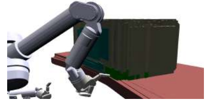
Figure 4.2: A decision region for pushing the button of a microwave. Each decision corresponds to putting the end-effector at a particular position and moving forward. For each decision, there are many poses of the microwave for which it would succeed. Instead of finding fully localizing the microwave, our goal is to reduce uncertainty just enough to know a particular decision will succeed.
