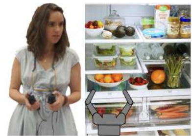
Figure 1.2: Assisting a user teleoperating a robotic arm requires dealing with uncertainty over their desired goal. Our work in shared autonomy is motivated by tasks like these, where clutter makes it impossible to infer the user's single goal until the end of execution.
