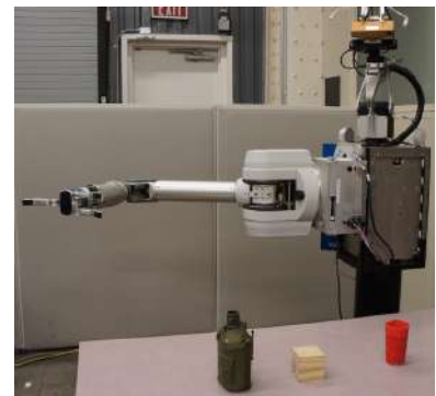
Figure 7.2: Our experimental setup for object grasping. Three objects - a canteen, block, and glass - were placed on the table in front of the robot in a random order. Prior to each trial, the robot moved to the configuration shown. Users picked up each object using each teleoperation system.
