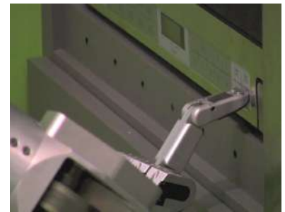
Figure 1.1: Pushing a small button on a microwave requires dealing with the uncertainty of object localization, noisy sensors, and arm kinematics. In tasks like these, we apply active information gathering to reduce uncertainty enough to achieve our goal.
