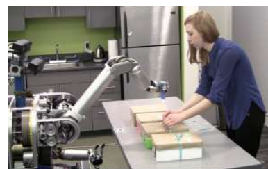
Figure 7.11: Participants performed a collaborative gift-wrapping task with HERB to evaluate our POMDP based reactive system against a state of the art predict-then-act method, and a non-adaptive fixed sequence of robot goals.
