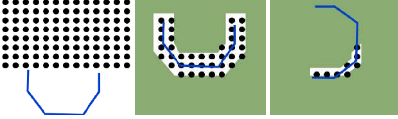
Figure 3.2: Touch-based localization as set cover. Each test-outcome pair amounts to covering (green area) the hypotheses (black dots) which do not agree, ruling out those hypotheses as they could not have generated that test-outcome pair. Maximize this coverage is adaptive submodular [GK11], rendering efficient greedy algorithms near-optimal.
