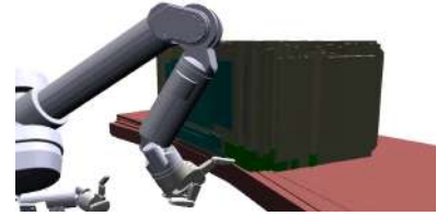
Figure 4.2: A decision region for pushing the button of a microwave. Each decision corresponds to putting the end-effector at a particular position and moving forward. For each decision, there are many poses of the microwave for which it would succeed. Instead of finding fully localizing the microwave, our goal is to reduce uncertainty just enough to know a particular decision will succeed.
