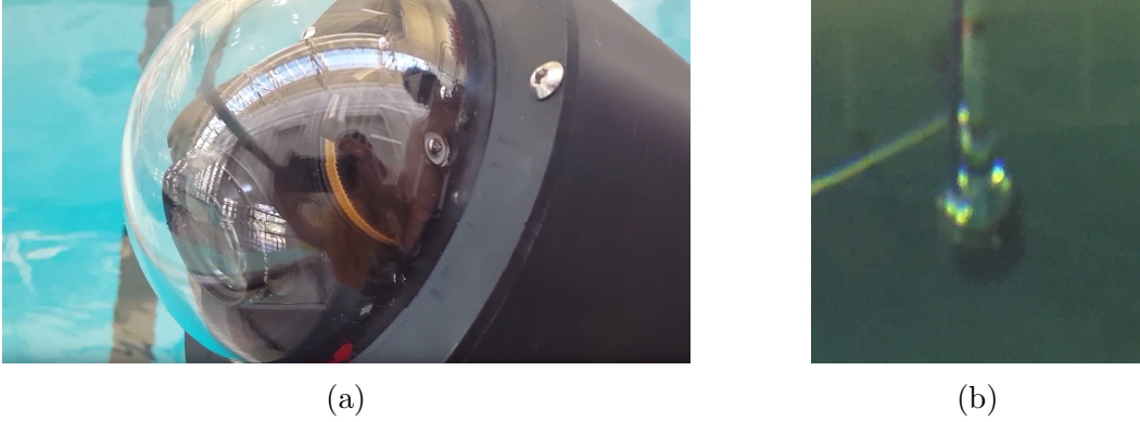
Figure 2.2: The PTZ camera used for the inspection system. The camera is contained within a waterproof enclosure that has a spherical housing. (a) Camera close-up. (b) Camera is attached to a pole and submerged. The tether shown here is a preventative measure for testing and is not part of the deployable system.
