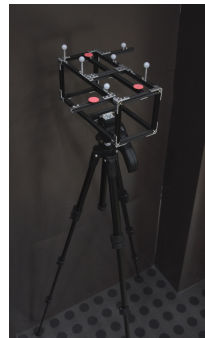
Figure 4.3: Subscale mockup system: (top) experimental setup shown with the subscale mockup of a reactor pressure vessel; (middle) camera image of the subscale system; (bottom left) external camera; (bottom right) subscale mockup of the inspection robot. Note the complete lack of visual texture on the structure.
