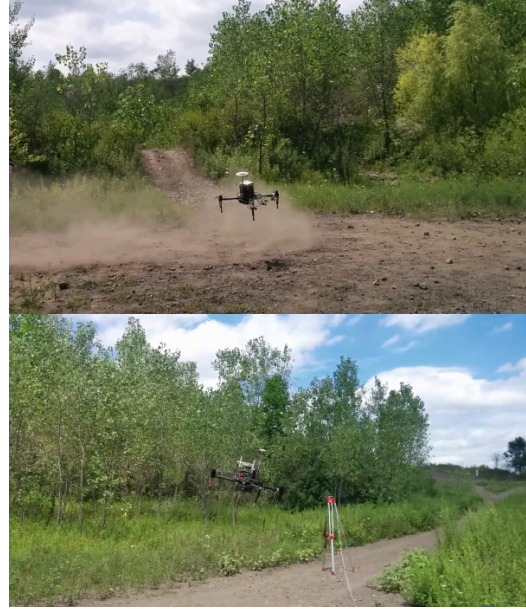
Fig. 1: Low altitude high speed navigation for MAVs. The robot makes a turn to go to the goal point and avoids the immediately seen obstacle.
