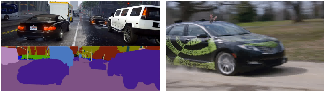
Figure 1.2: Demonstrations of the end-to-end approach on autonomous navigation applied to (a) the realistic simulator (GTA V), and (b) the full-size vehicle by NVIDIA[3].
