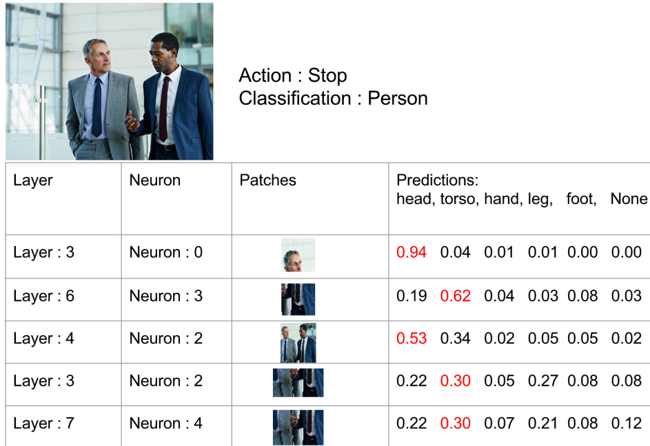
Figure 4.6: APPLE sorts the labeled patches by confidence to present to a human in order to explain the CNNs image classification and corresponding action (important patches are selected using Weight Matrix Sum measure)
