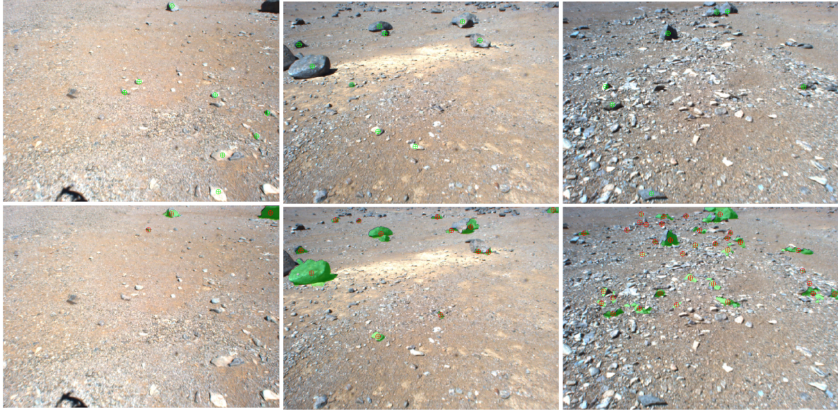
Figure 9: Image set B : Top row, ground truth centroids in green, bottom row, detected rocks shaded green with RHoCS-computed centroids in red.
