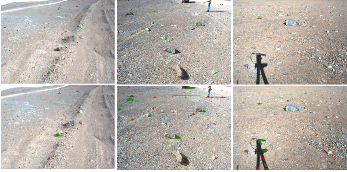
Figure 22: Image set D : Top row, ground truth centroids in green, bottom row, detected rocks shaded green with RockNet-computed centroids in red.
