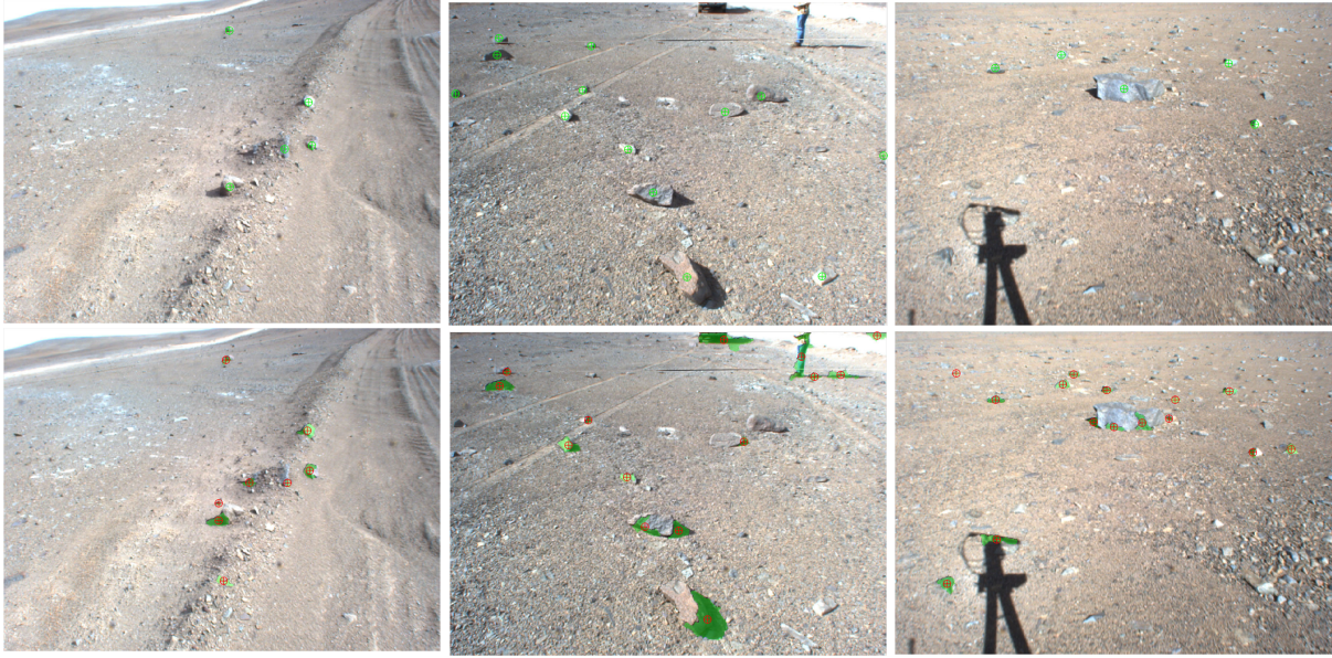
Figure 11: Image set D : Top row, ground truth centroids in green, bottom row, detected rocks shaded green with RHoCS-computed centroids in red.
