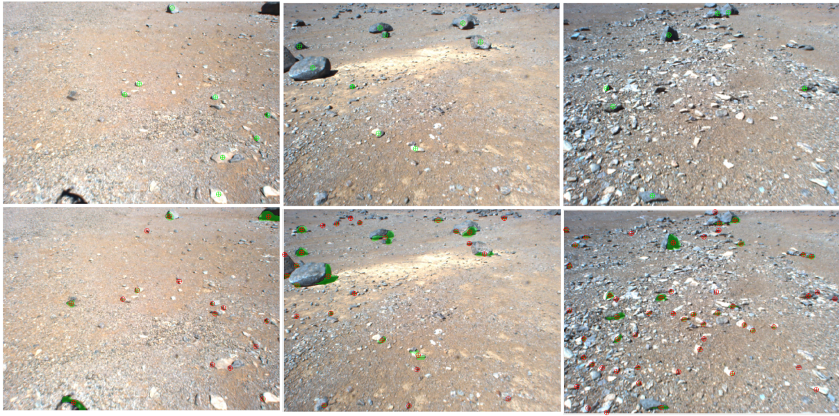
Figure 20: Image set B : Top row, ground truth centroids in green, bottom row, detected rocks shaded green with RockNet-computed centroids in red.
