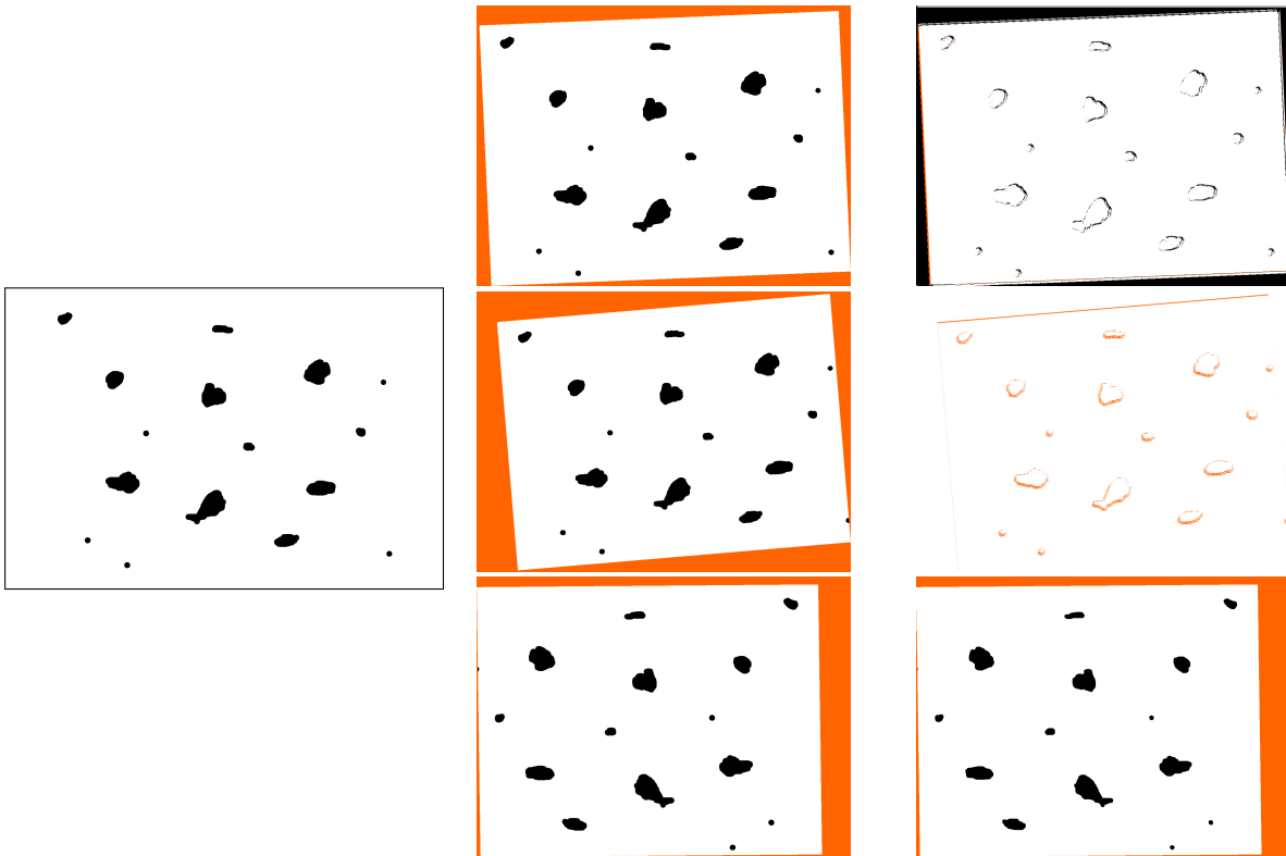
Figure 13: Simple synthetic rock images to test various CPN architectures. Left shows original image, middle shows affine augmentation inputs, and right shows the resulting labels for three different CPN architectures. As demonstrated by the poor results at the top and middle images of the right column, even simple synthetic images require some tuning of the CPN architecture.
