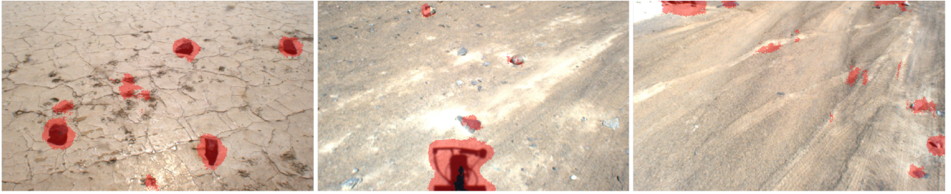
Figure 6: TextureCam results with failure cases in the top 5% most confident rock classifications.
