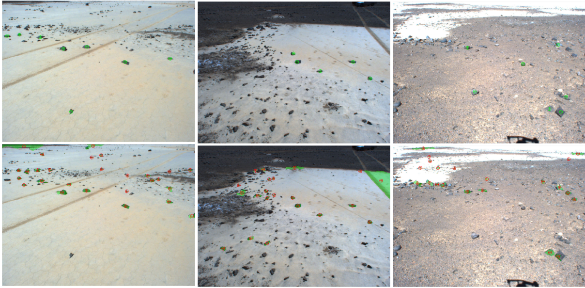
Figure 8: Image set A : Top row, ground truth centroids in green, bottom row, detected rocks shaded green with RHoCS-computed centroids in red.
