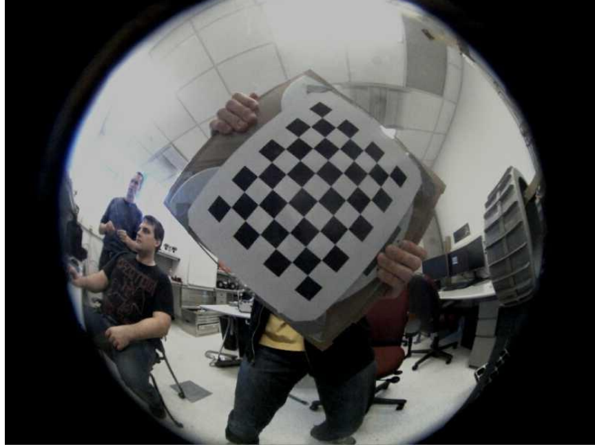
Figure 8: Example Calibration Test Pattern Image
