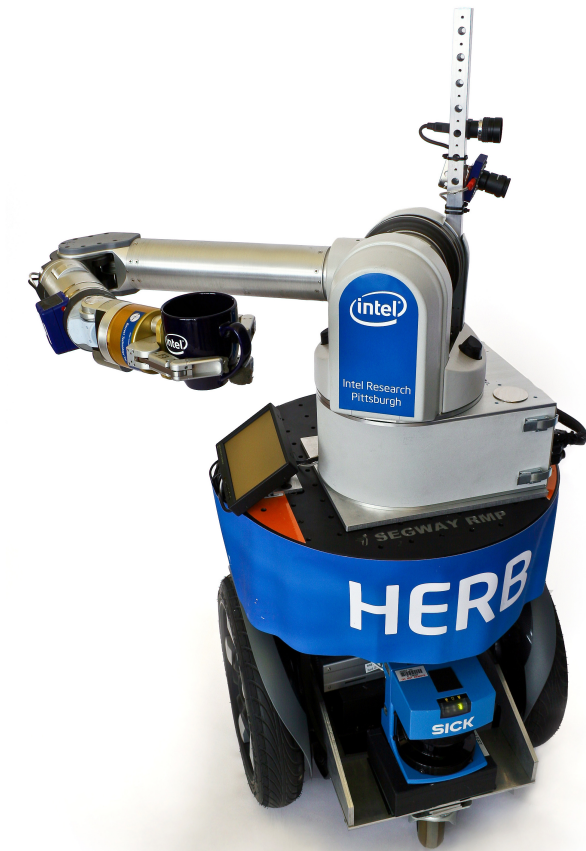
Figure 3.1 HERB is a mobile manipulation platform comprising a WAM arm and Segway base.
