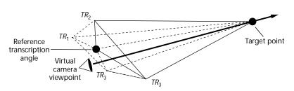
Figure 7. Selection of supporting transcription angles. Given a reference transcription angle, we determine the supporting angles by first enumerating the neighboring angles  $(TR_i)$  of the reference and then forming the triangles containing the reference transcription angle and two of the neighbors. The triangle pierced by the line of sight of the virtual camera determines the supporting angles.
