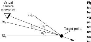
Figure 6. Selecting the reference transcription angle.  $\theta_i$  is the angle between the virtual camera's line of sight and the line joining the target point with the position of the transcription angle TR<sub>i</sub>. We select the transcription angle TR<sub>i</sub> with the smallest angle  $\theta_i$  as the reference transcription angle.
