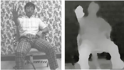
(a) intensity image (b) corresponding disparity map Figure 2: An example scene and its range image
