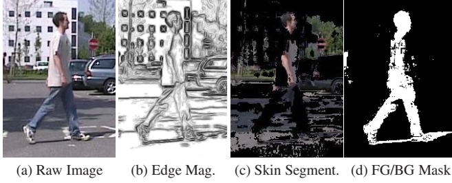
Figure 5: A sample image (a) and three low-level visual cues (b)–(d) combined in the imaging model.
