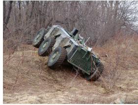
Figure 7: Crusher hybrid electric vehicle used in field tests
