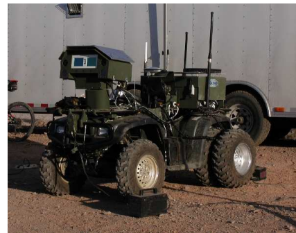
Fig. 1. Unmanned ground vehicle used during the phase-II. This vehicle is based on an ATV chassis. The laser radar, mounted on a pan-tilt head, is visible at the front of the vehicle. The rear box contains the different computers necessary to control the autonomous behavior of the robot.
