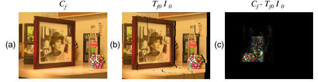
Figure 7: Color updating illustration. (a) Observed view . (b) Forward warped frontal color . (c) Difference image, which provides color estimates for the rear layer when warped back to the reference view .
