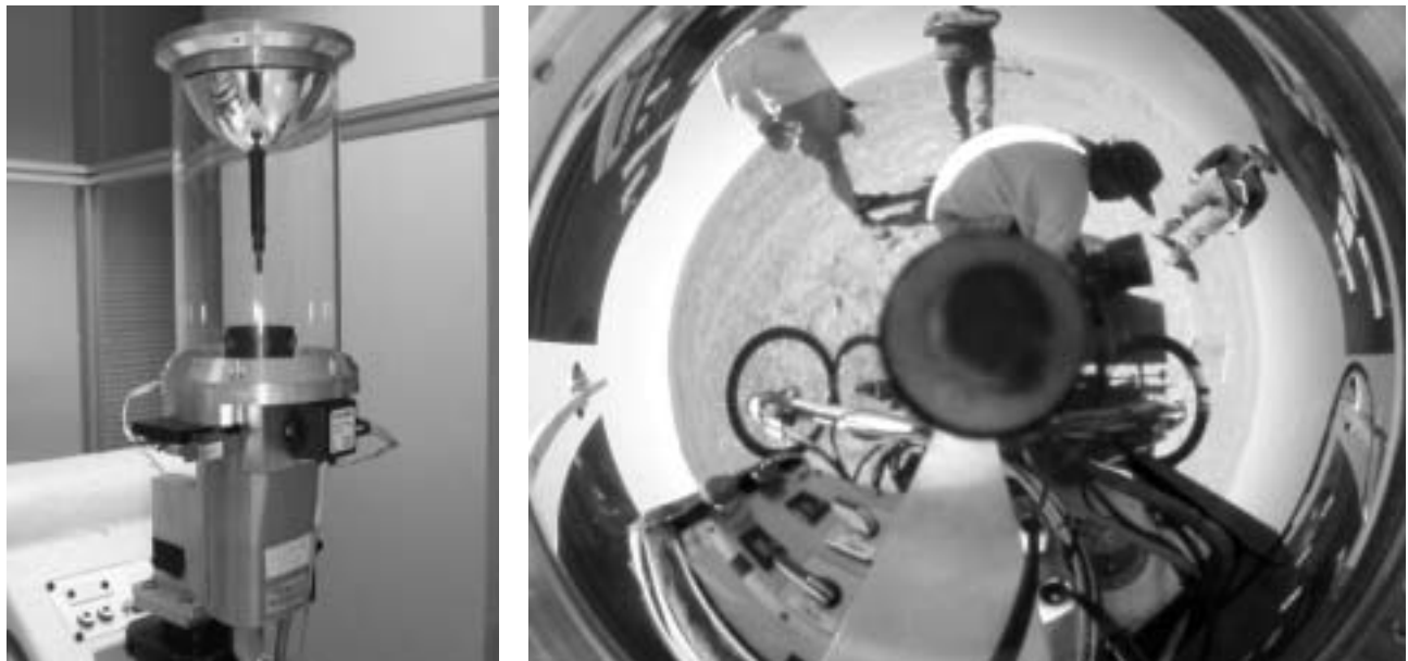
Fig. 4. Left: an omnidirectional camera consisting of an IEEE 1394 camera attached to an equiangular mirror by a rigid cylinder. The accelerometer and one rate gyro are visible, attached to the rig below the cylinder. Right: an omnidirectional image produced by this design.
