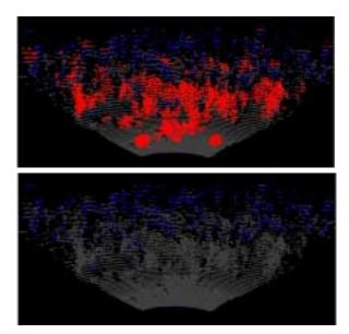
**Figure 8.** The picture on the left shows flat terrain covered with grass and weeds. The terrain is completely traversable. The top right shows the traversability classification for this terrain using geometric data only. The red areas are false obstacles; the blue areas are unknown. The bottom right shows an updated classification taking "drivability" metrics into account. Note that the vegetation has been eliminated as obstacles.
