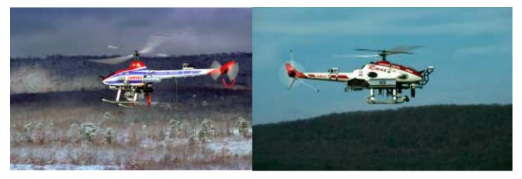
Figure 3. The Yamaha R50 autonomous helicopter (left) and the Yamaha RMAX autonomous helicopter (right).
