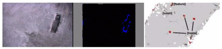
**Figure 9.** The left image shows a photo of a coffin-sized hole taken from the FE at 10 m altitude. The center image shows the hole detected as an obstacle using stereo vision. The right image shows several holes the size of an excavator bucket detected with ladar from the FE at 25 m altitude.
