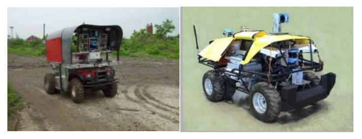
Figure 1. First (left) and second (right) generation UGV test vehicles based on the Honda Rubicon ATV platform.
