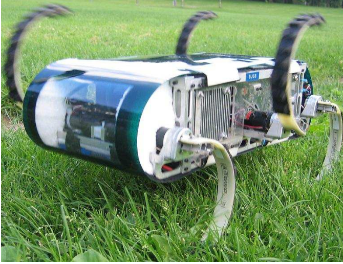
Figure 4.1: RHex’s configuration features six C-shaped compliant legs that rotate around the hip. Different leg synchronization schemes produce different behaviors, such as walking, jogging and stair climbing.
