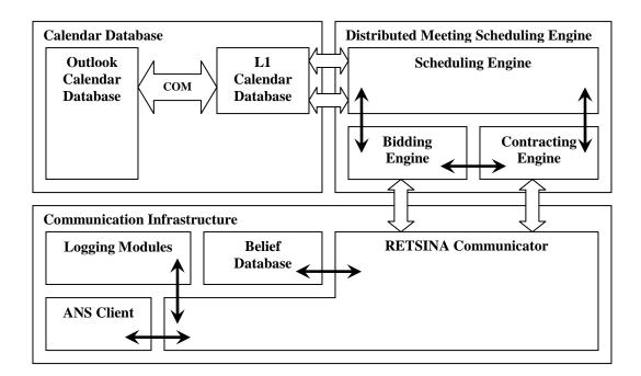
Figure 3: RCal Modular Block Diagram
