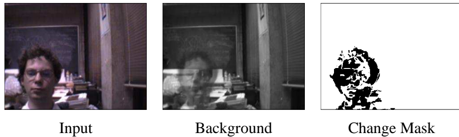
Figure 6.5: Examples of the input image, the background image which is a decaying average of the input, and the change detection mask, used to limit the amount of the image searched by the neural network. Note that because the person has been stationary in the image for some time, the background image is beginning to include his face.
