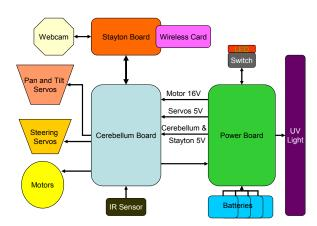
Fig. 4. PER electronics schematic.
