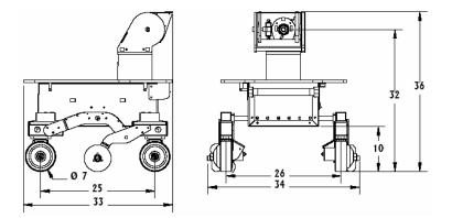
Fig. 3. PER dimensions in centimeters.
