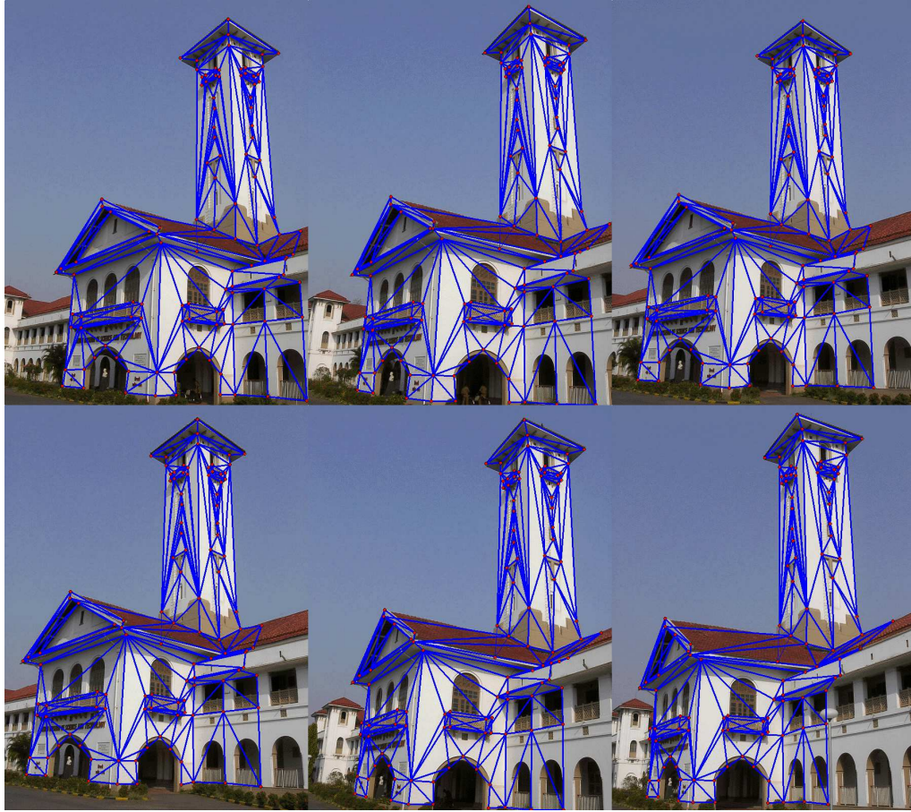
Fig. 6. Six out of the eighteen images used to extract the position of the points are superimposed with the initial mesh. The points, which are used as vertices of the mesh, do not exactly correspond to real corners and the edges thereof do not correspond to edges of the actual surface.
