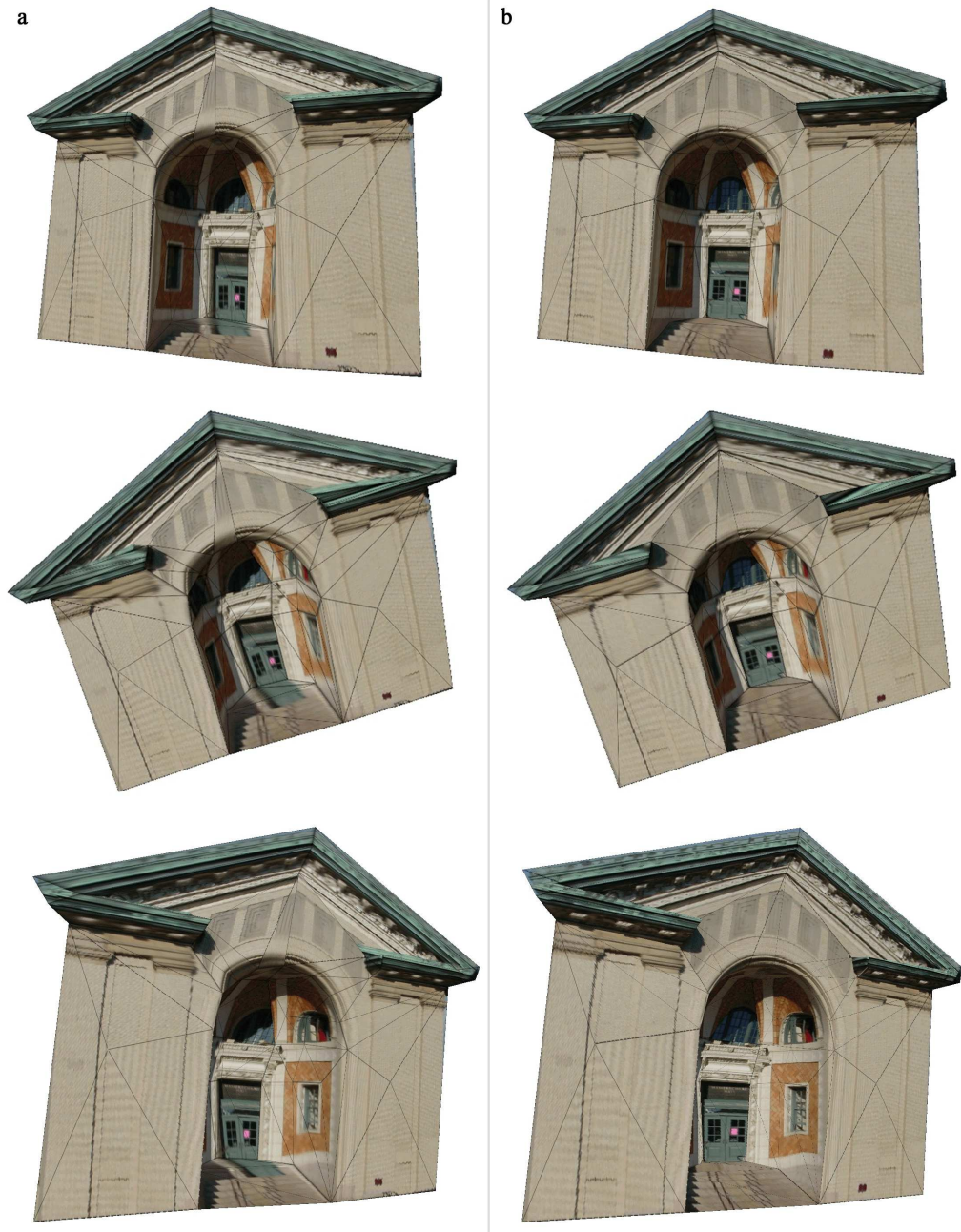
Fig. 14. Shown in column a are views of the model for the initial position of vertices. Views corresponding to the EigenFaired model are in column b on right. Note that the initial model has textural artifacts especially prominent along the curved dome, facade edges, and door steps. Artifacts in 3-D modeling are prominent when models are viewed from oblique angles. Renderings of the EigenFaired model, on the other hand, are devoid of artifacts.
