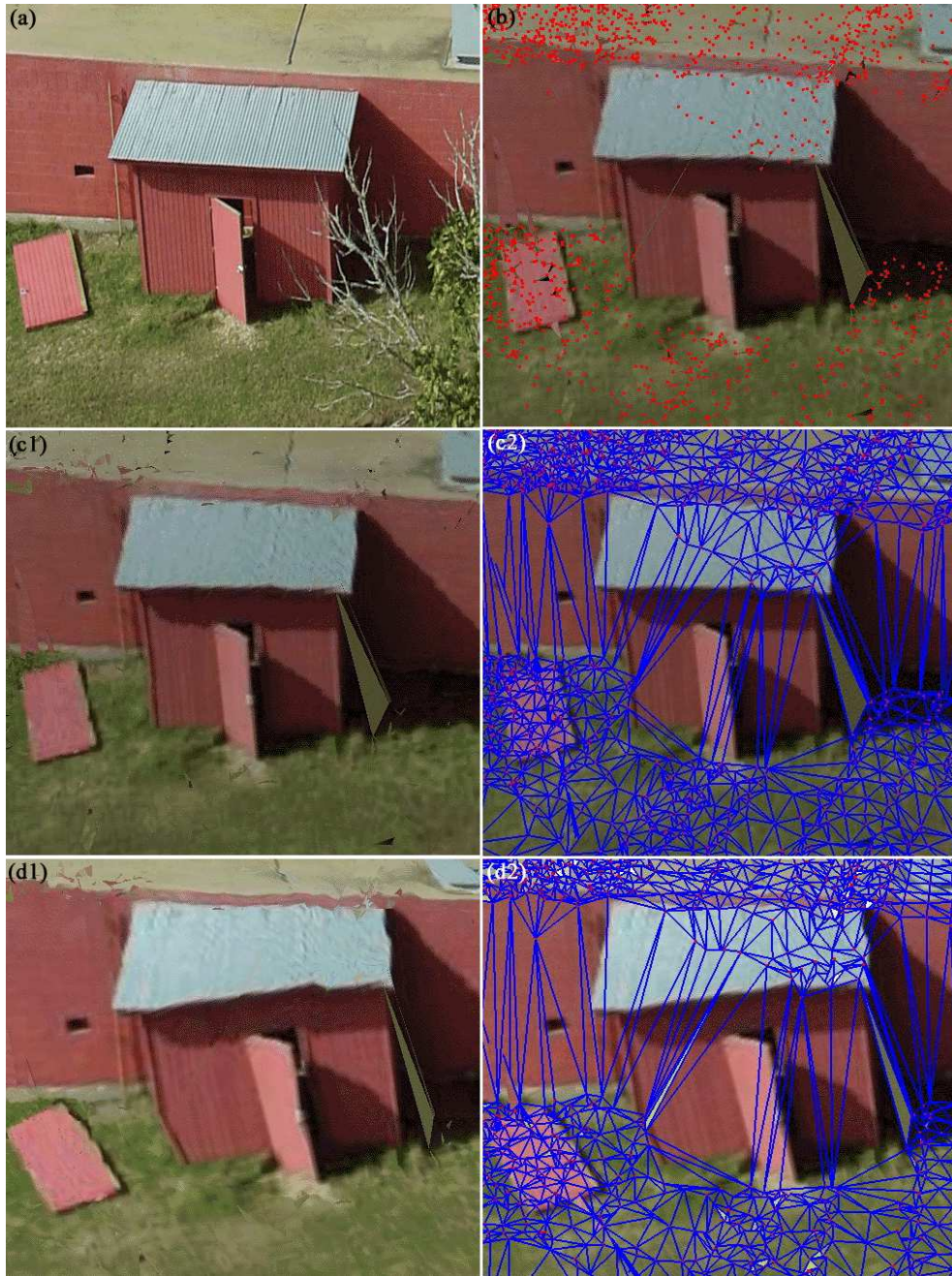
Fig. 3.1. Model-based Rendering: (a) The original image as observed from a particular viewpoint, (b) Depth data superimposed on the rendering of the modeled surface from the same viewpoint, (c1) Rendered image of the model, (c2) The underlying mesh of the 3-D model, (d1) Rendered image from a slightly different viewpoint, and (d2) The corresponding mesh as viewed from the new viewpoint.
