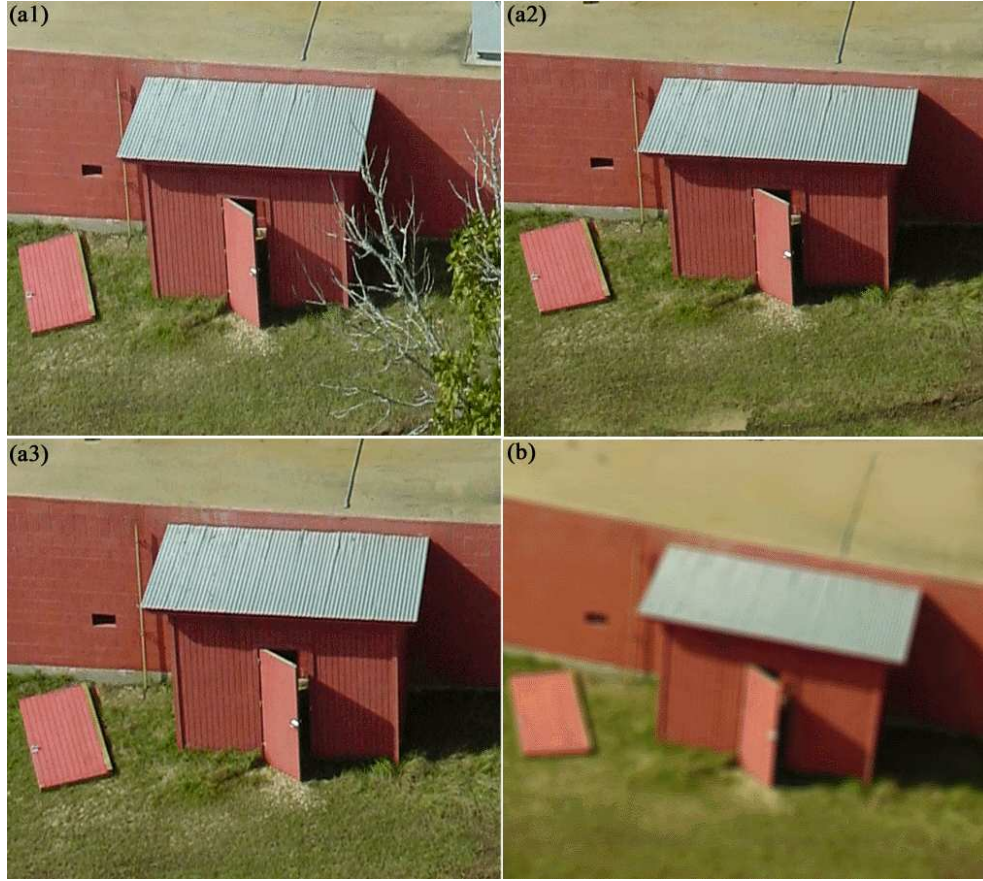
Fig. 3.2. View-based Rendering: (a1, a2, a3) Three from a set of 8 images taken from different viewpoints, and (b) Image rendered from a new viewpoint using the image-based rendering technique proposed by (Fitzgibbon et al., 2003). The new viewpoint is around 16 degrees apart from the closest viewpoint in the image sequence.
