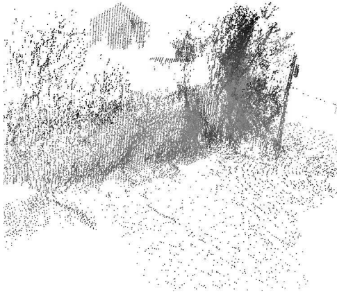
Fig. 2.4. Noise is caused by quantization of a 3-D point-coordinate as well as inaccuracy in spatial distribution of the mesh density (topology).
