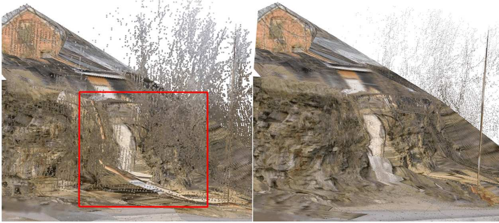
Fig. 5. A thin and elongated face occludes small areas of larger triangles of the mesh when viewed from a particular direction. On the left is a model where each face of the mesh is texture-mapped using a single image. In self-occluding models, “smears” of texture inconsistent with the model often get mapped onto the mesh. A better idea is to texture-map a face by the image cell that has the lowest distance-from-feature-space (DFFS). The artifacts are not present in the latter case.
