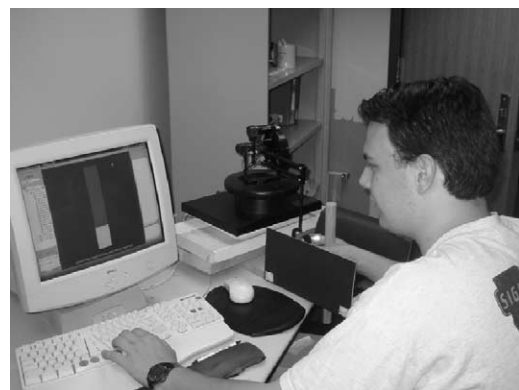
Fig. 1. Our experimental setup. A subject was seated on a chair facing a computer monitor that displayed the visual feedback bar of force/position. His index finger was secured to the robot with a finger splint. Forces were issued tangential to the finger's semicircular trajectory. The forearm was restrained to minimize shifting. The subject's view of his hand was occluded during the experiment with an opaque cover (not shown).
