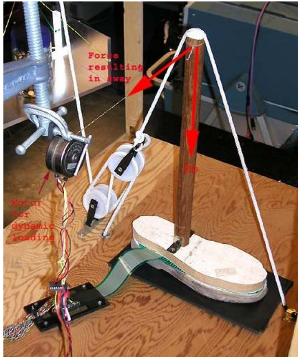
Figure 2. Detail of the foot, leg, static and destabilizing loading mechanisms.
