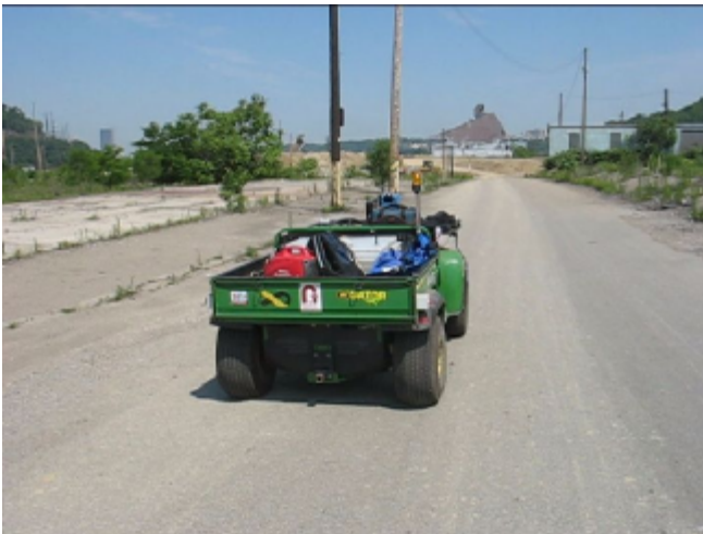
Fig 8. E-gator autonomous vehicle used for testing and electric poles used for localization at test site. The vehicle equipped with wheel encoders and a KVH E- core 1000 fiber-optic gyro for dead reckoning, and a tilting SICK ladar and onboard computing for navigation and obstacle detection
