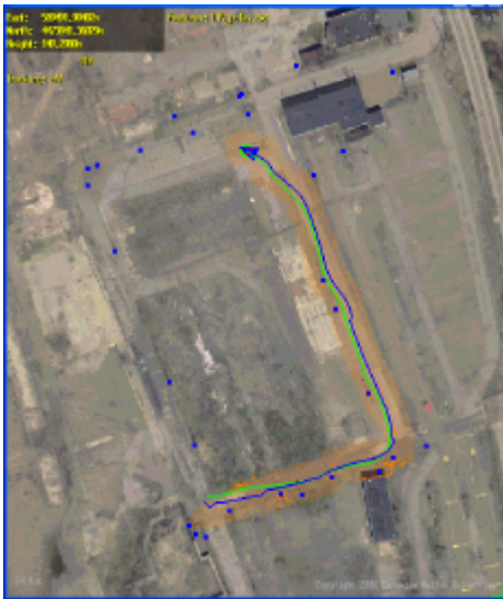
Fig 10. Path planned and executed without GPS. Blue dots show the location of landmarks. The blue line is the position estimate of the Kalman filter on the robot and the green line is the position reported by a WAAS differential GPS with accuracy of approximately 2 meters (for reference only).
