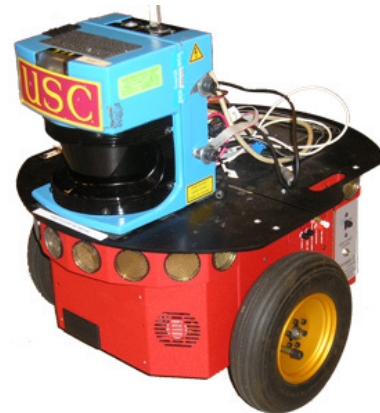
Figure 1: The Pioneer 2-DX mobile robot used in this study, with a SICK scanning laser range finder mounted on top.
