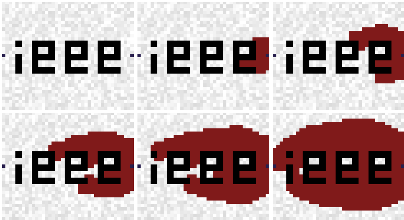
Figure 3. Example of Focussed Dynamic Programming in action. The initial state is on the far left with the goal on the far right (both darkly shaded). In red (darkly shaded) are the states examined during the course of the algorithm. The sequence runs from left to right, top to bottom.
