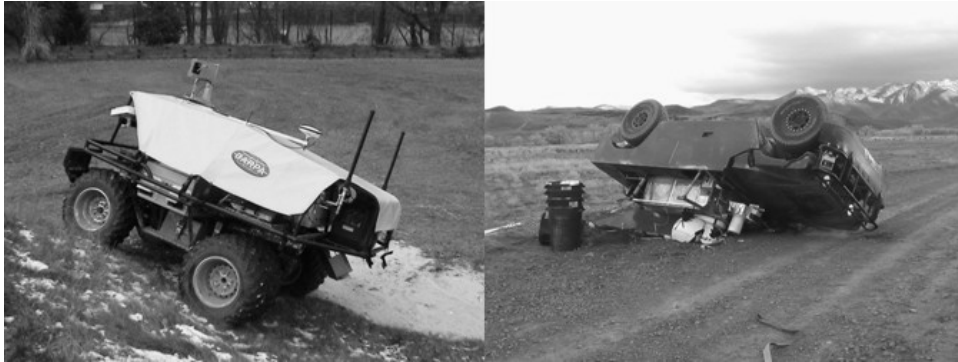
Fig. 1. Robot rollover events at CMU in 2004. [Left] The rough terrain vehicle "Yellow" shown suffered a 360 degree rollover due to soil failure on a long slope. [Right] The Grand Challenge vehicle called Sandstorm rolled during high speed testing due to several factors including high lateral acceleration during cornering.
