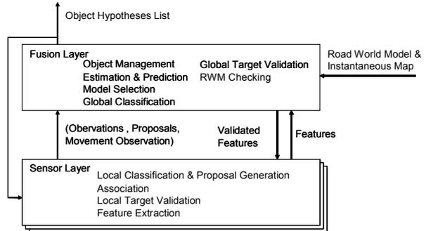
Fig. 3: Software Architecture for Object Tracking
