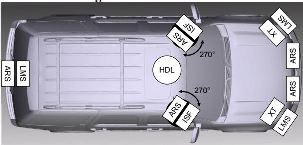
Fig. 2: Sensor Configuration for Object Tracking [8].
