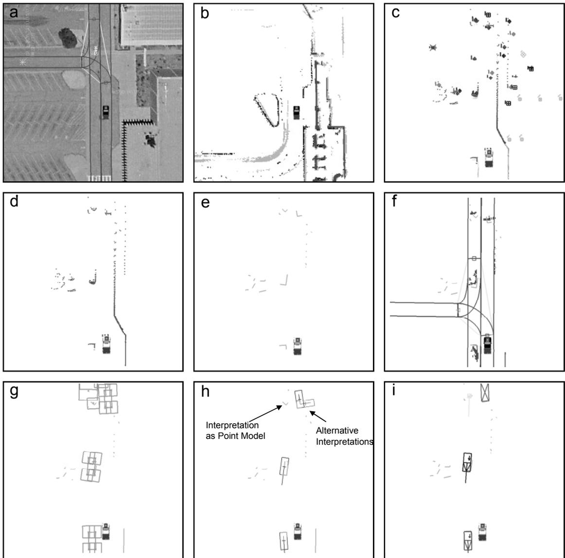
Fig. 4: a) Road Structure b) Static Map; Illustration of object tracking algorithm: c) Raw data (diamonds represent radar detections, dots originate from laser scanners) d) only laser scanner data e) features extracted from laser scanner data f) feature validation against road structure and instantaneous obstacle map g) data association h) interpretation of features and proposal generation i) Model selection and update of state estimation (see [8]).
