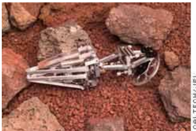
Figure 2.5: A single degree of freedom hopping robot that self-oriens itself before propulsion (Courtesy: Caltech/JPL).
