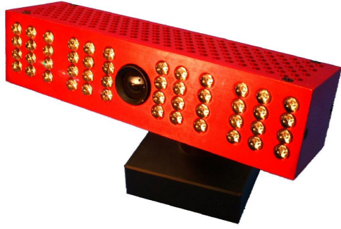
Figure 1: The CSEM SwissRanger2 flash lidar device
