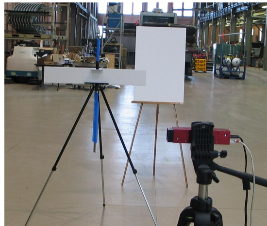
Figure 4: Experimental setup to determine the effect of mixed pixels on flash lidar devices
