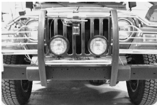
Figure 1: The omni-camera is mounded in front of the vehicle – NavLab11.
