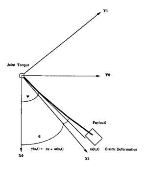
Figure 1: The One Link Flexible manipulator
