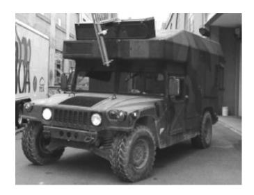
Fig. 14. The autonomous vehicle (HMMWV) used for our experiments. The vehicle is equipped with stereo vision, inertial guidance and GPS positioning.
