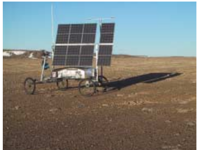
Figure 1: The Hyperion rover, for which TEMPEST generated sun-synchronous routes. Note the vertical solar array and long polar shadow
