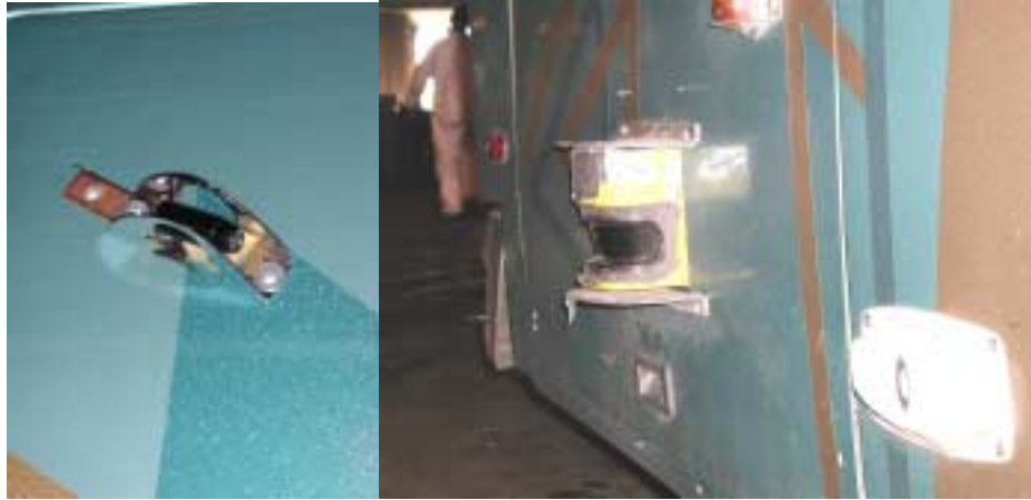
Figure 18 - The installed camera and laser scanner
