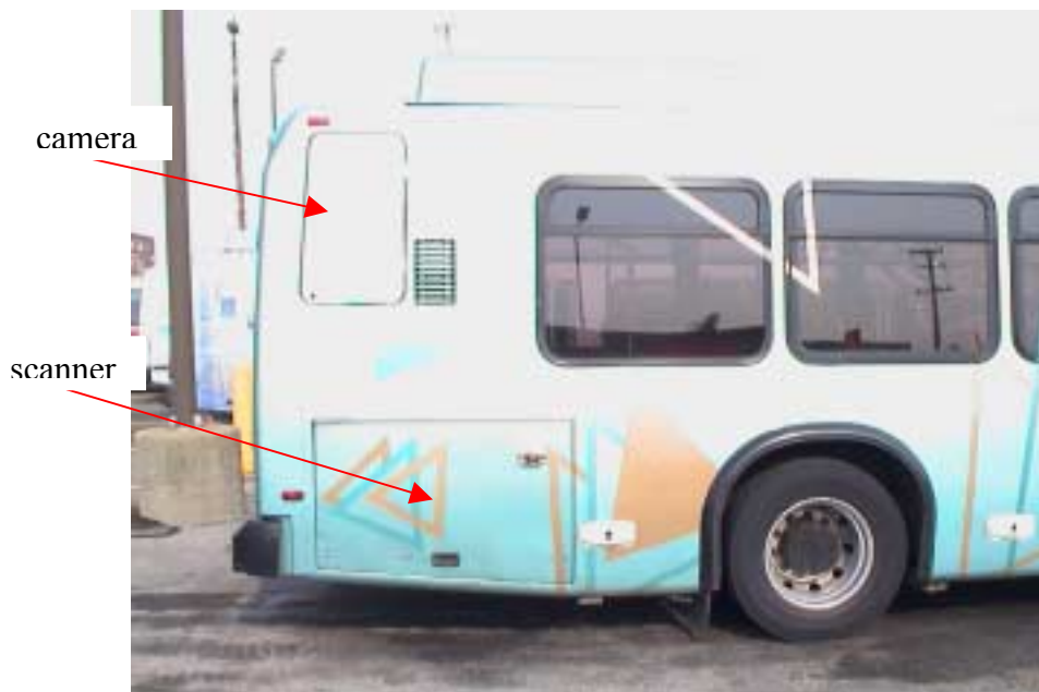
Figure 17 - Bus before the installation of the sensors. The arrows point to the locations where the camera and the laser scanner will be installed.
