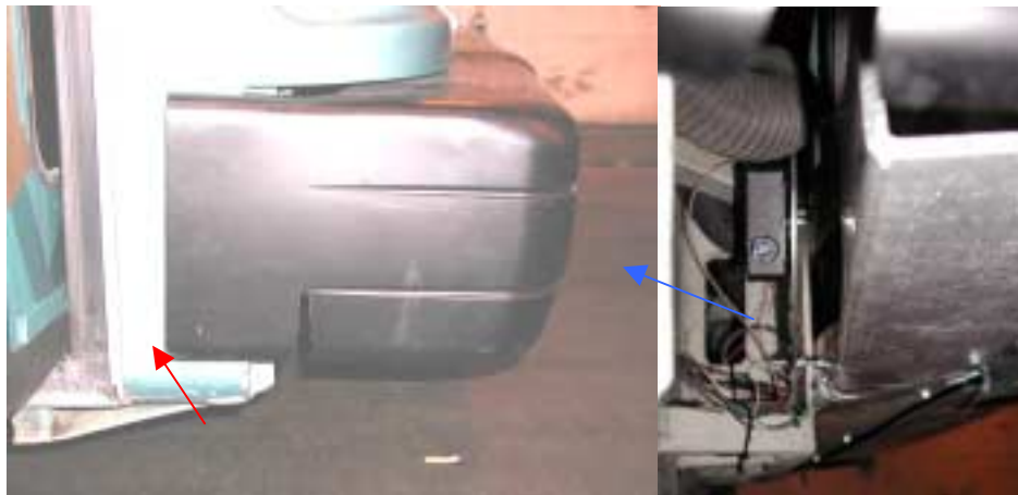
Figure 19 - In the left the front bumper of the bus is shown with a small slit (red arrow) where the laser light exits. On the right the underside of the bumper is shown with the laser of the curb detector visible (blue arrow).
