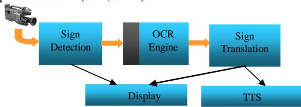
Fig. 8. System architecture.
