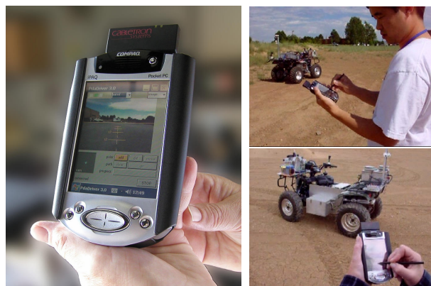
Figure 1: Left , PdaDriver (version 3) on a Compaq iPAQ; right , Remote driving with PdaDriver
