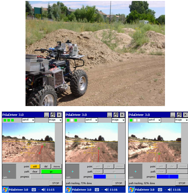
Figure 8: Top , AATVIL driving on a dirt road; bottom left to right , Image mode display sequence (color camera): designated path with three waypoints, first-half of path achieved, approaching final waypoint.
