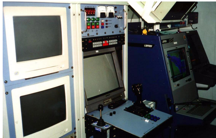
Figure 51. Direct teleoperation interface (International Submarine Engineering, Ltd.)
