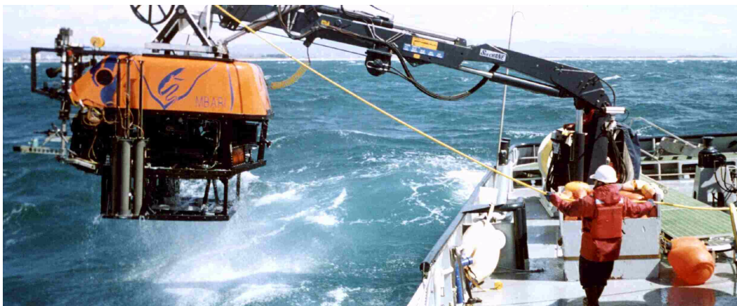
Figure 50. A work-class ROV designed for drilling support and oceanographic research (International Submarine Engineering, Ltd.)
