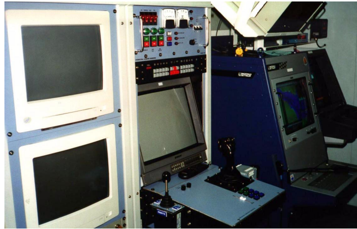
Figure 3. Direct teleoperation interface (International Submarine Engineering, Ltd.)
