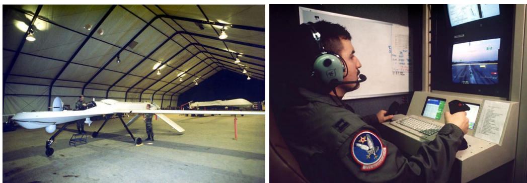
Figure 44. Left, Predator (USAF Air Combat Command); right, Predator control station (USAF Air Combat Command).
