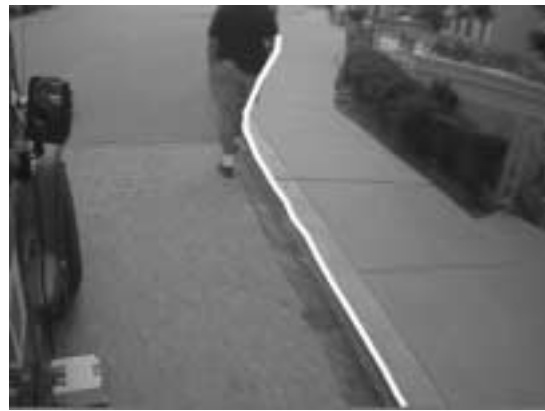
Figure 11: Erroneous curb detection caused by a pedestrian in front of the curb.
