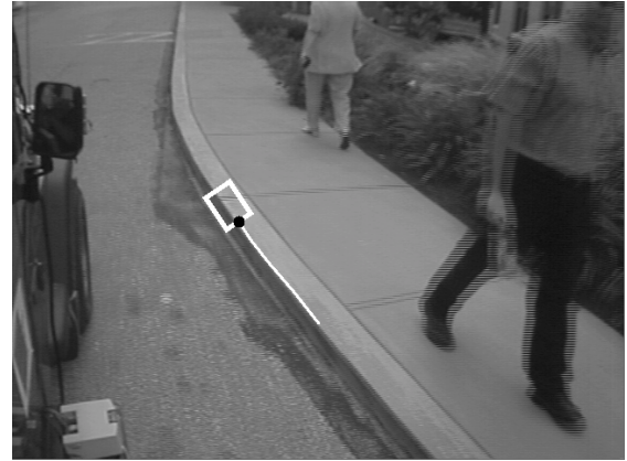
Figure 7: Interest zone (white rectangle) in the image with current curb detection (black dot) and the track (white line).
