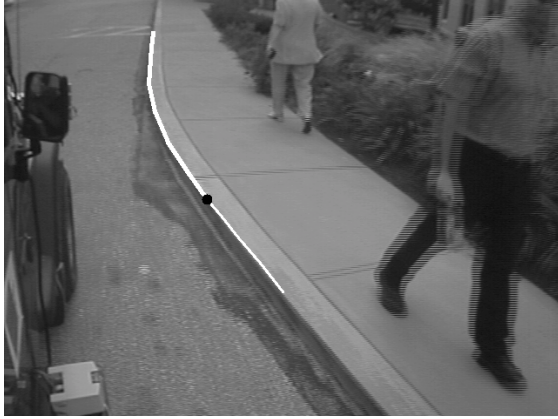
Figure 8: Detected curb alongside and in front of the vehicle.
