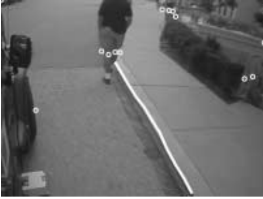
Figure 12: Video data with obstacle information. The raw image is the same as in Figure 11; the data from the laser scanner is indicated as white circles. The detection of the curb is correctly terminated when it reaches the obstacle.
