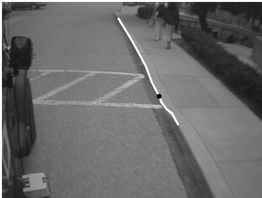
Figure 9: Curb ramp on the side of the vehicle. The laser line striper cannot see the curb along the ramp, it is followed by the video detection instead.
