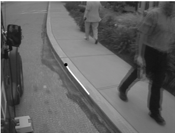
Figure 6: Current detection (black circle) and track (white line) of the curb viewed by a camera mounted on the side of the vehicle.
