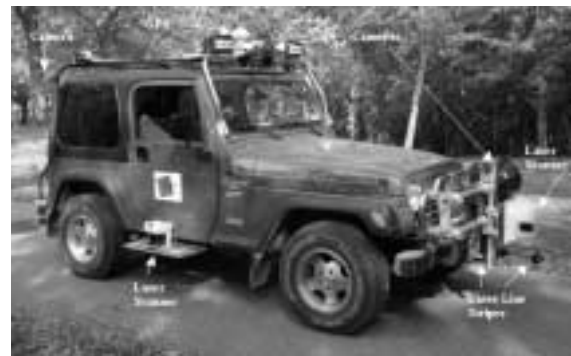
Figure 1: The experimental vehicle NAVLAB11 as a platform for various sensors.
