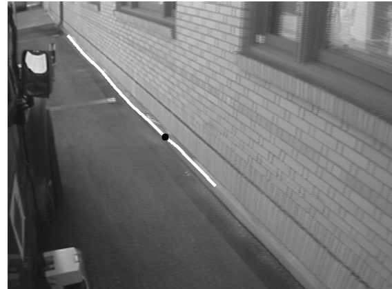
Figure 15: Detecting the edge of an outdoor brick wall.
