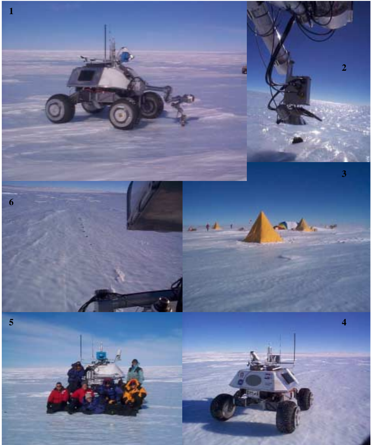
Clockwise from upper left: Nomad's manipulator deployed to a meteorite; a close view of Nomad's wrist examining a meteorite; the Elephant Moraine January 2000 base camp; Nomad in autonomous search mode; the expedition team; the view from Nomad's high-resolution camera
