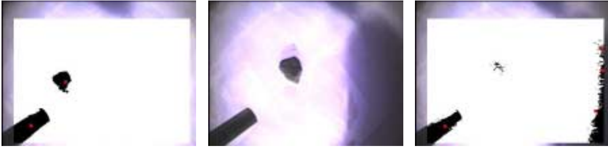
Figure 10. From left to right: segmented image from first visual servoing step, raw image from second step (notice the robot's shadows on the right) and segmented image from second step
