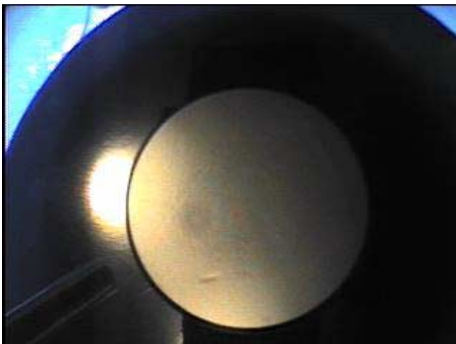
Figure 9. Spectrometer calibration target seen from arm camera
