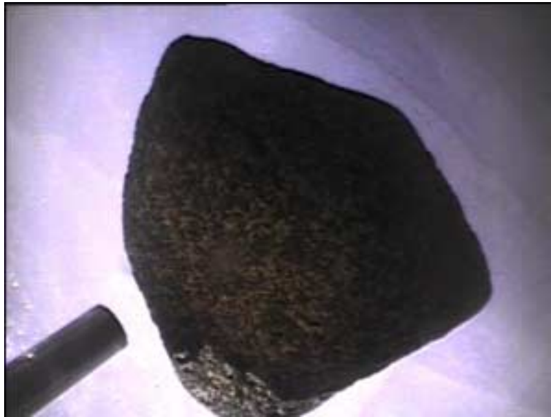
Figure 17. Top: reflectance spectrum of ID #0 (spectrometer head > 2 cm from rock), bottom: arm camera image as spectrum was being taken
