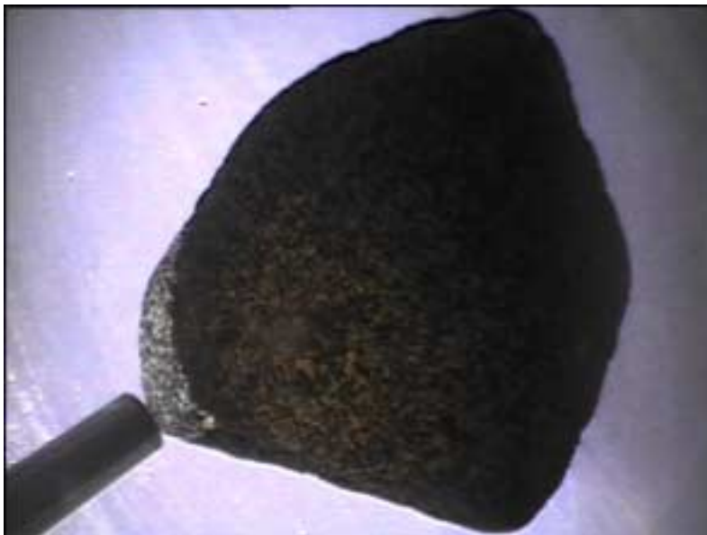
Figure 18. Top: reflectance spectrum from ID #1 (spectrometer head 1 to 1.5 cm from rock), bottom: arm camera image as spectrum was being taken
