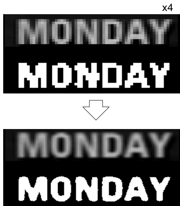
Figure 13: High Resolution Image Creation Original image/binary image, high resolution image/binary image
