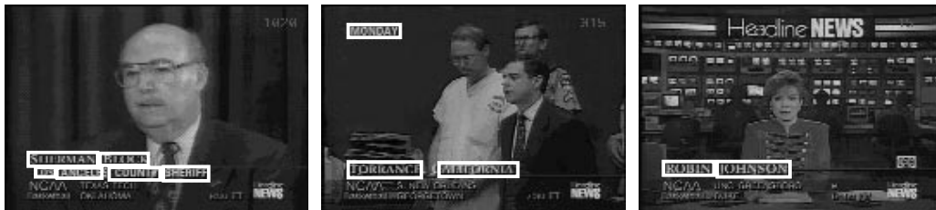
Figure 11: Text detection results with various images. CNN Sports Ticker portion (bottom portion) was eliminated from processing.
