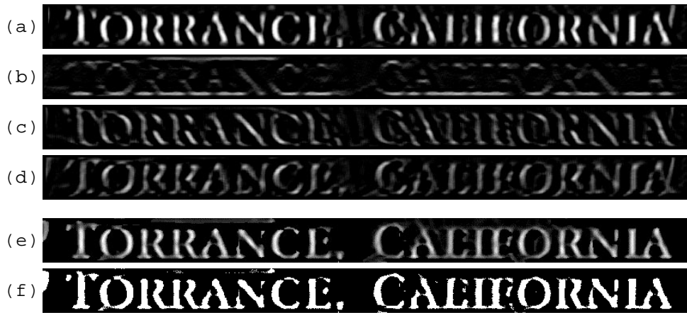
Fig. 8. Result of character extraction filter. (a)0°. (b)90°. (c)-45°. (d)45°. (e)Integration of four filters. (f)Binary image.
