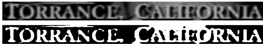
Fig. 5. Result of sub-pixel interpolation and multi-frame integration (upper). Binary image (lower). Pixel size is 813 \times 56 .
