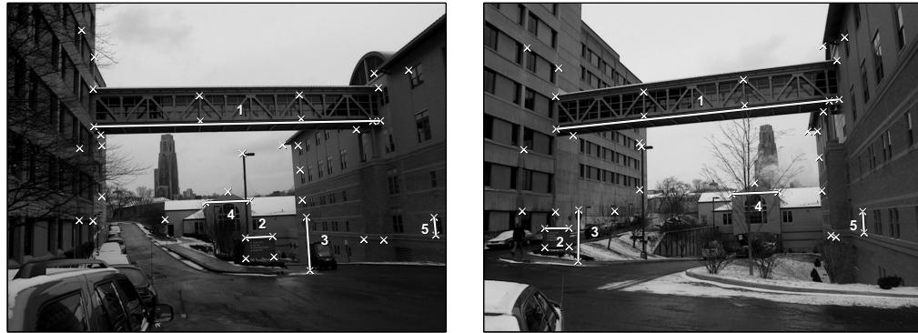
**Fig. 4.38.** The two end-images from a seven image sequence of a bridge. Our goal is to estimate the length of the bridge, marked with line 1, and to do this we measured the lengths of lines 2 through 5.
