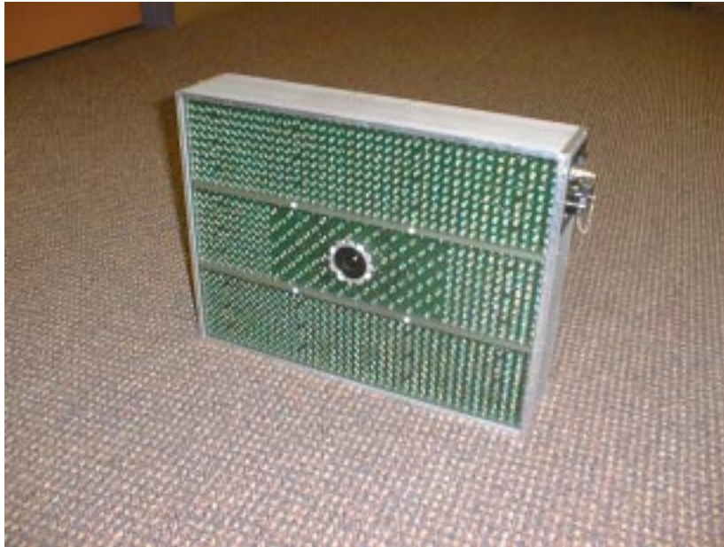
Figure 20: Lighting and Imaging Module. This device is a custom solution for low power, engineered lighting. Its slimline form factor renders it mountable underneath vehicles. Resulting light levels are uniform over the floor.
