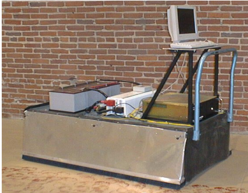
Figure 22: Mapping Rig. This custom engineered vehicle is used to create mosaics. It couples a downward looking camera for acquiring imagery with an odometry system for estimating relative motion between images.
