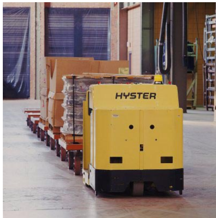
Figure 23: Tug AGV. This automated guided vehicle is one of several with mosaic-based positioning installed.
