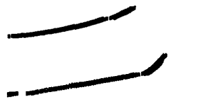
Figure 4. A classification of the laser reflectance scans in Figure 2, based on the absolute value of an edge operator. Black pixels indicate a potential obstacle.
