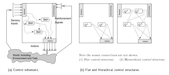
Figure 1 Schematic of control architectures: (a) sensory, action and reinforcement signal configuration for a learning control system and (b) control architectures: (1) flat structure and (2) hierarchical structure. Note:  $Q^{?}$  represents behaviors and the sensory connections in (b) have been removed for clarity.
