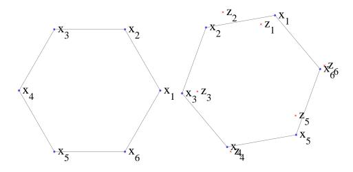
Figure 1: Left: A 2D model shape, defined by points on a circle with radius 1. Right: Measured feature points. The true rotation is 70 degrees, measurement noise  $\sigma = 0.2$ .
