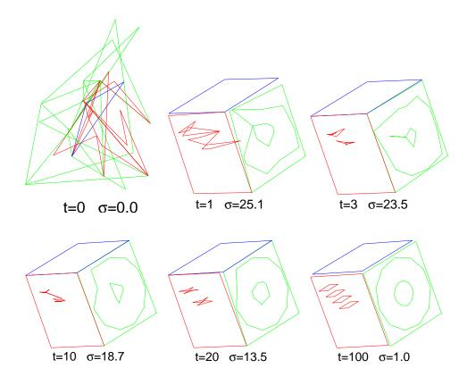
Figure 6: Starting from a random guess for the structure (t=0) we recover gross 3D structure in the very first iteration (t=1). As the annealing parameter  $\sigma$  is gradually decreased, successively finer details are resolved (iterations 3,10,20, and 100 are shown).
