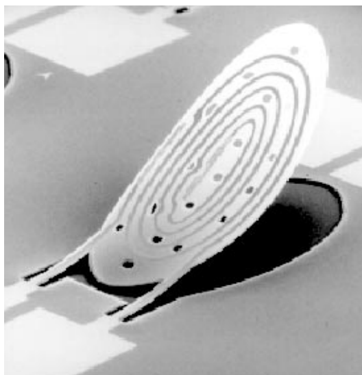
Figure 4. Example of an “active surface” MEMS device. This one is a tiny “flap”; many flaps working together could potentially reduce drag on an airplane wing as suggested in Figure 1, or position a part for assembly.
